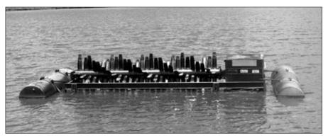
Figure 5. A 10-hp electric paddlewheel aerator.
