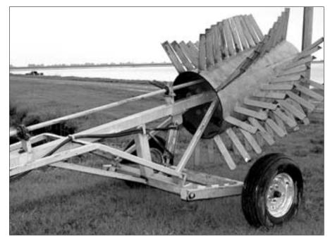
Figure 3. A sidewinder paddlewheel showing the orientation of paddles on the hub.
